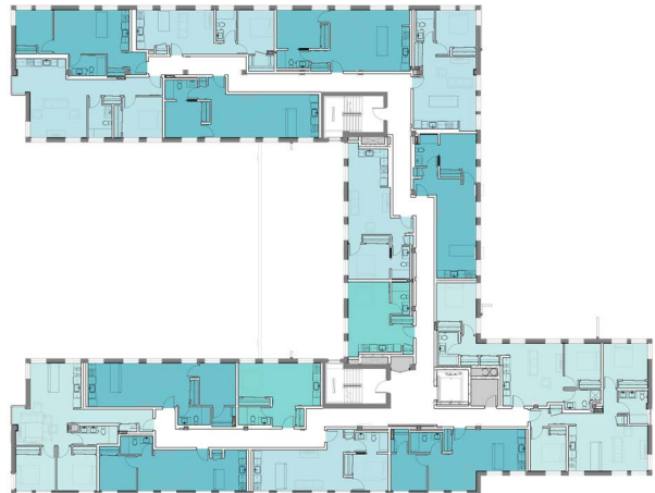
Carver Hall new typical floor plan Shifting the corridors to either side of the beamline allowed for additional space within each apartment.
